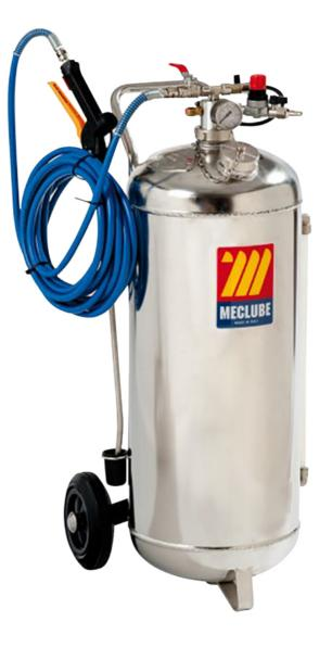
Equipment suitable for the nebulisation of detergents with foaming device. When they are filled with liquid for 3/4 of their capacity and air is put inside at 6-8 bar they work automatically without any continuous link to compressed air.
