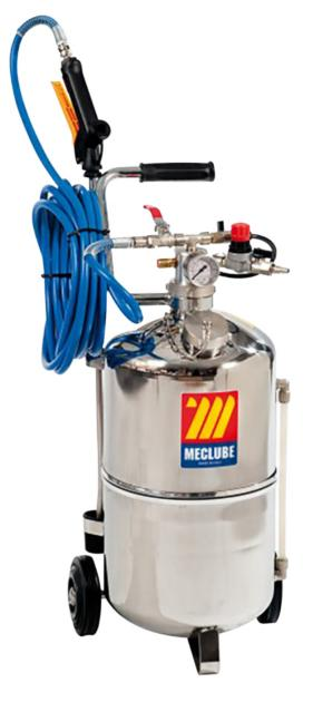
Equipment suitable for the nebulisation of detergents with foaming device. When they are filled with liquid for 3/4 of their capacity and air is put inside at 6-8 bar they work automatically without any continuous link to compressed air.
